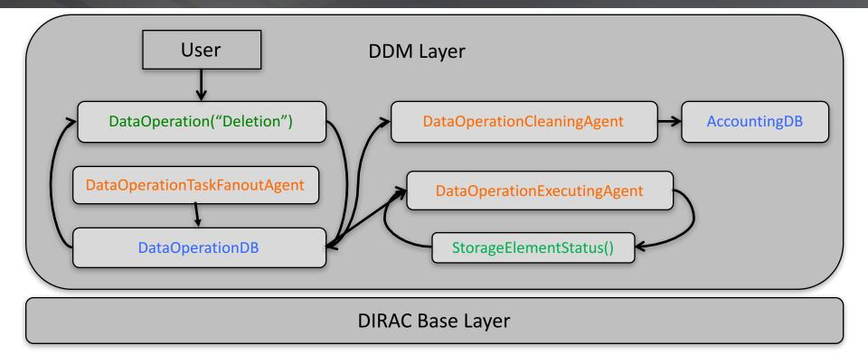
DDM by design does not delegate deletion of files to base DIRAC to avoid race conditions on data files
