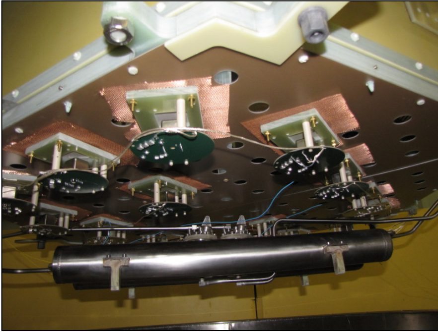
Criotec Liquid Recirculation system attached to the bottom of the TPC frame
