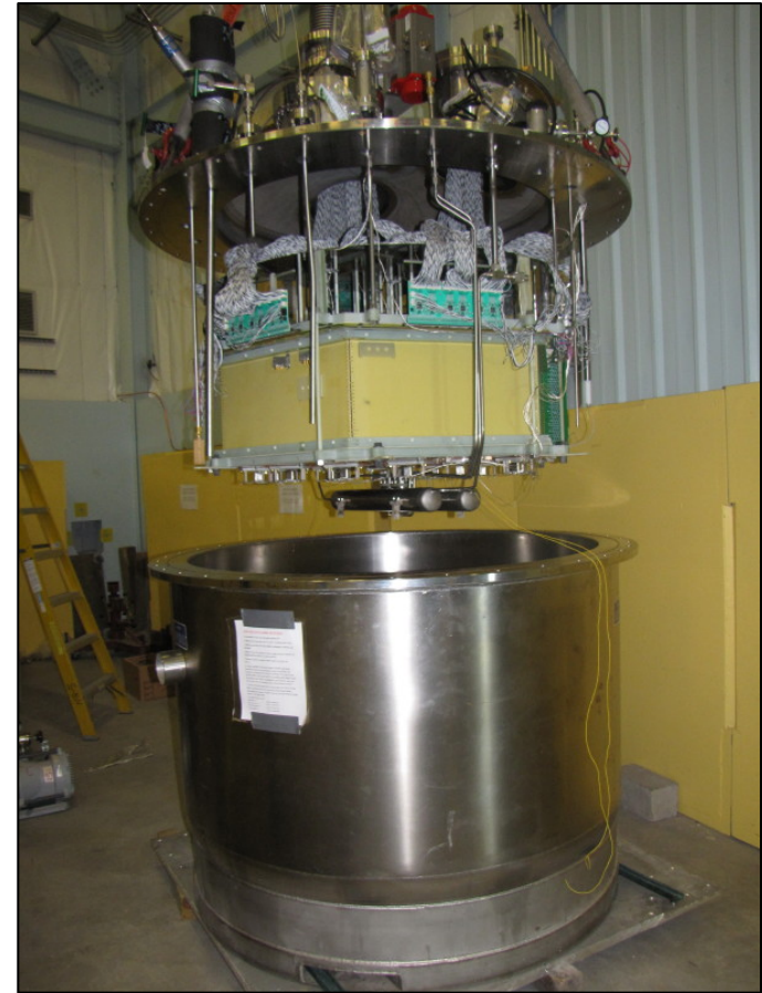
TPC being lowered into the Mini-CAPTAIN cryostat before filling in May 2017
