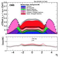
L1 Residual scale factors (<sup>Data</sup>/<sub>MC</sub>) used to correct for differences in PU offset in data and MC.
