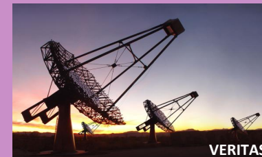
Imaging Atmospheric Cherenkov Telescope (IACT) 50 GeV – 20 TeV
