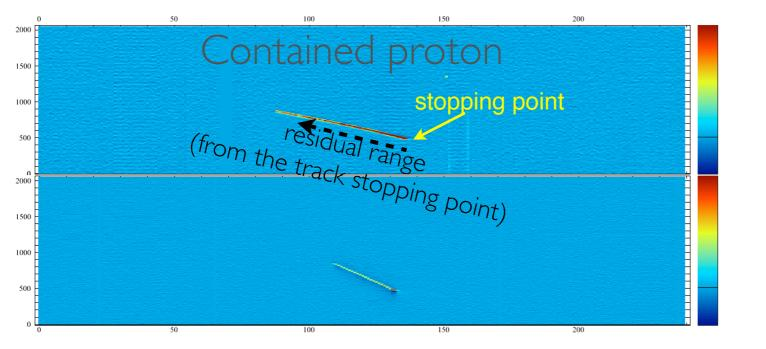
The energy loss as a function of distance from the end of the track is used as a powerful method for particle identification.
