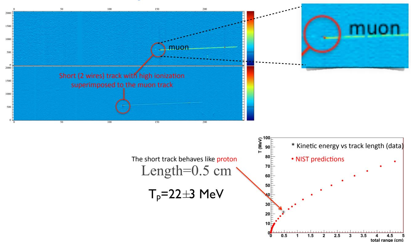
ArgoNeuT proton threshold: 21 MeV Kinetic Energy
