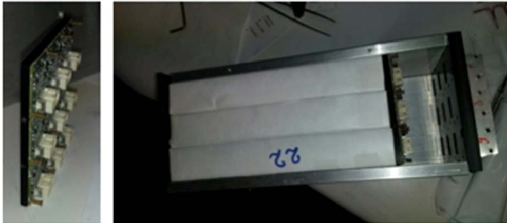
Figure 3.5. Amp-HV prototypes and assembling in the pure CsI crystals matrix.
