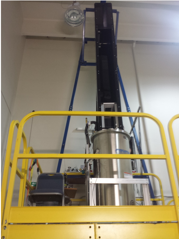
Mechanical test apparatus for mechanical tests of up to 4 PDs in LN2 bath
