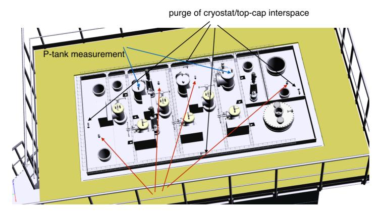
4 KF ports connected to the top-cap IS which are free.
