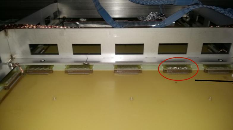
We realize one connector of the CRP was not soldered. David soldered it in place because was not possible to remove it. After this we found only 3 dead channels: 2 signal and 1 ground channels.
