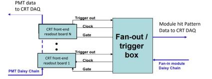
Data stream contains 32 bit timestamp can be used for data merging offline, only when a proper bit is asserted in the main data stream.
