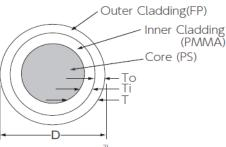
Cladding Thickness<sup>2</sup>:T=2%(To)+2%(Ti) =4% of D Numerical Aperture : NA=0.72 Trapping Efficiency : 5.4% Prototypes tested in beam line, readout with <u>CITIROC</u>: an analogue front-end ASIC made by Omega Microelectronics (CNRS-IN2P3-Ecole Polytechnique) [I. Ortega et al, proceedings to be published]
