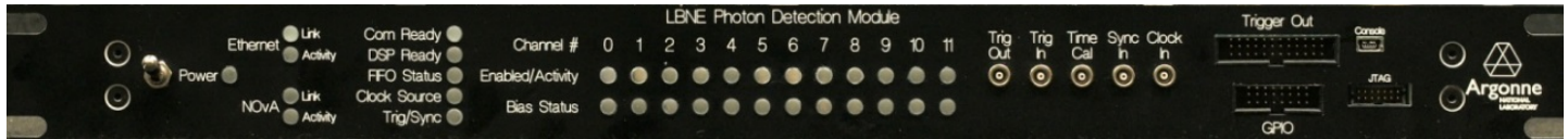
Figure 2-1: Picture of the front panel of the SSP.
