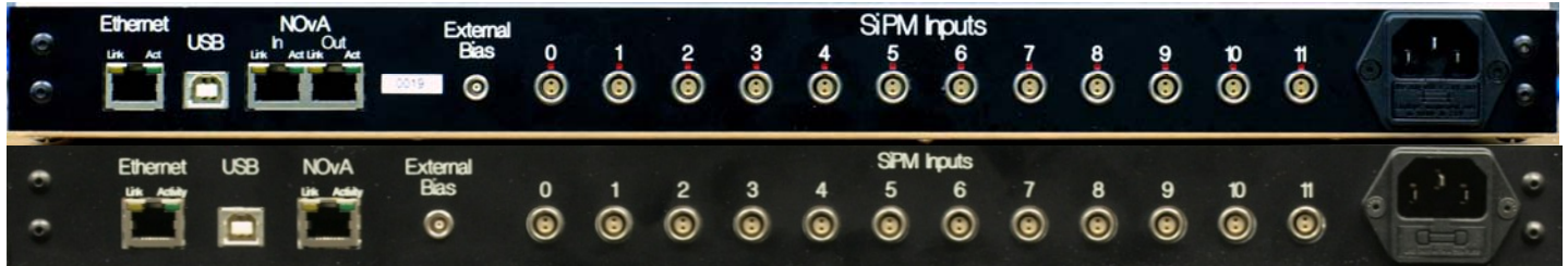
Figure 2-7: Picture of the rear panel of the SSP. (Rev A-Top, Prototype-Bottom)
