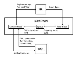
Figure 1: Block diagram showing interfaces of Boardreader to DAQ and SSP, and inter-thread communication within the Boardreader.
