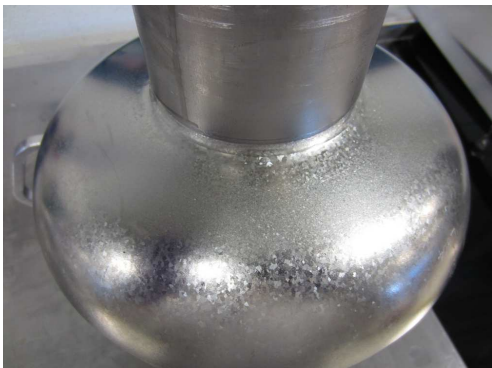
FIG. 4. Grain growth in AES011. The cavity was fabricated from material with \sim 100 \mu\text{m} sized grains, some of which grew to the few mm-scale after only a few UHV furnace cycles at 800^\circ\text{C} that were each 3 hours long or shorter.
