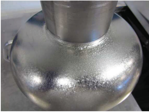
Figure 5: Significant grain growth observed in AES011.
