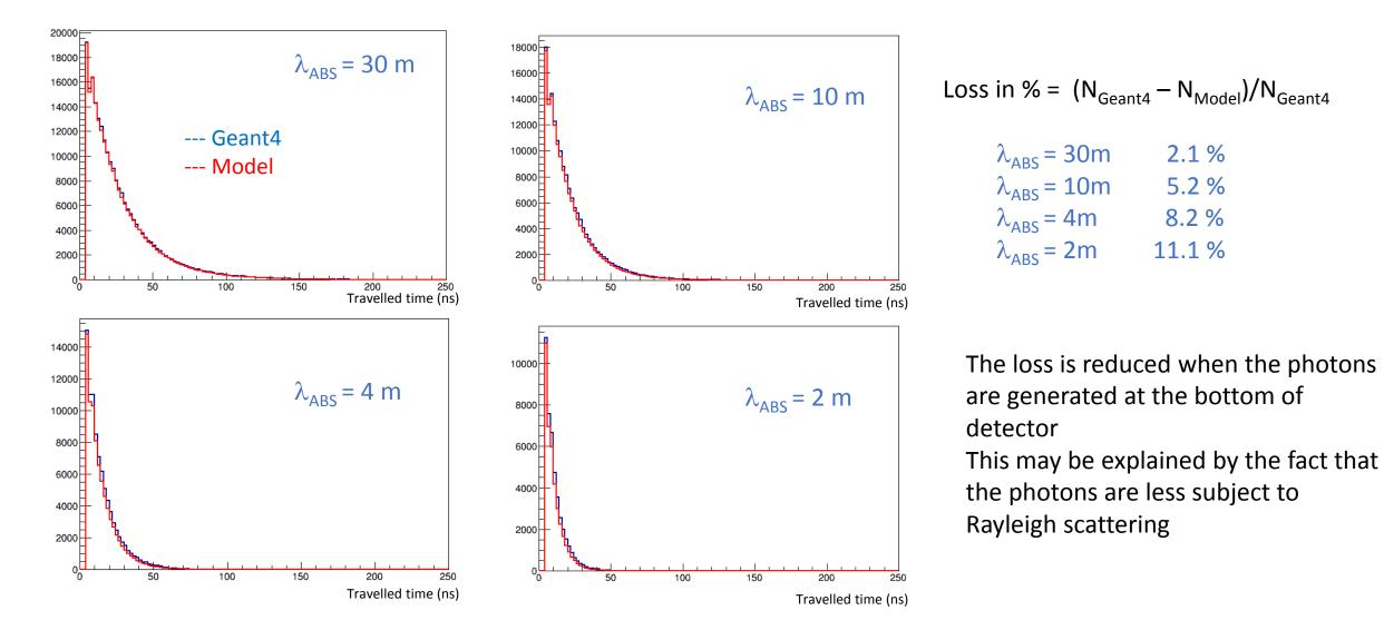
Comparison between Geant4 simulation results including absorption processus and a classical absorption model with an exponential exp(-travelled distance/  $\lambda_{ABS}$ )
