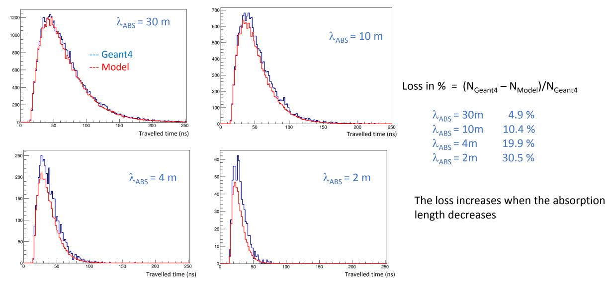
Comparison between Geant4 simulation results including absorption processus and a classical absorption model with an exponential exp(-travelled distance/  $\lambda_{ABS}$  )
