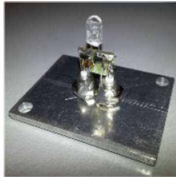
370 nm LED with pulser circuit
