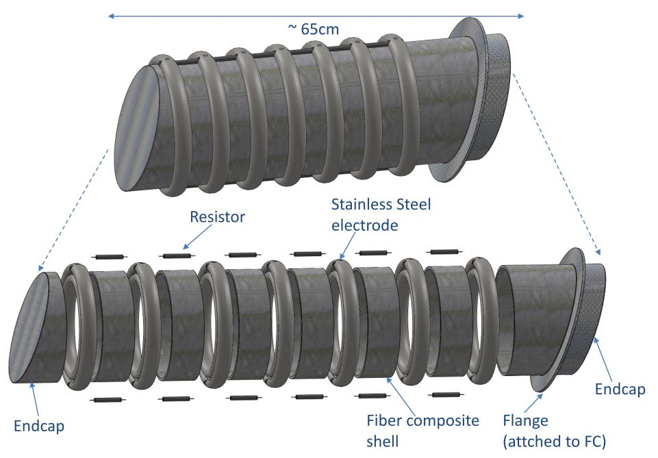
Sections are bonded using cryogenically-rated adhesive to ensure leak-free joint
