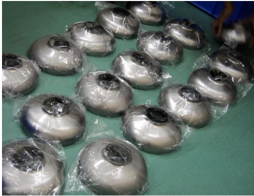
Machined half cells of five-cell SCRF cavity
