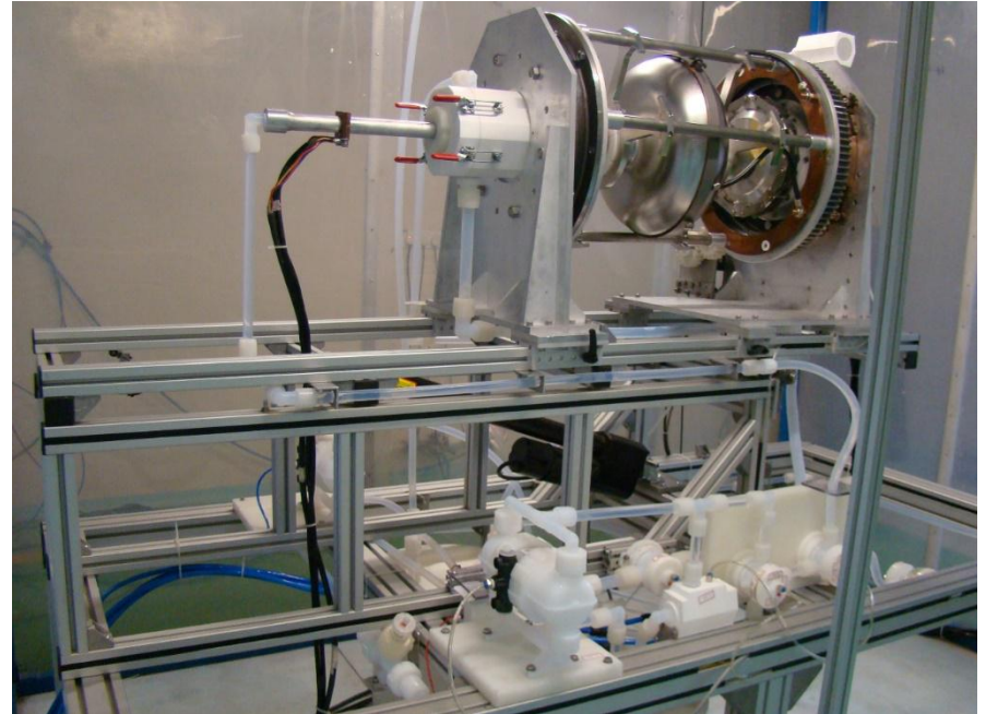
EP bench for 650 MHz Cavities
