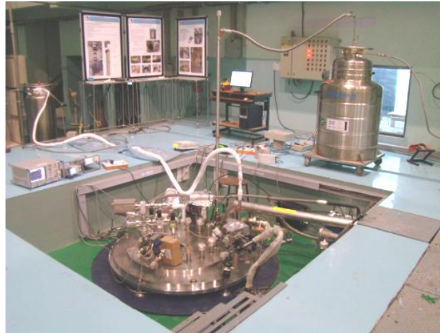
Transfer of liquid helium
