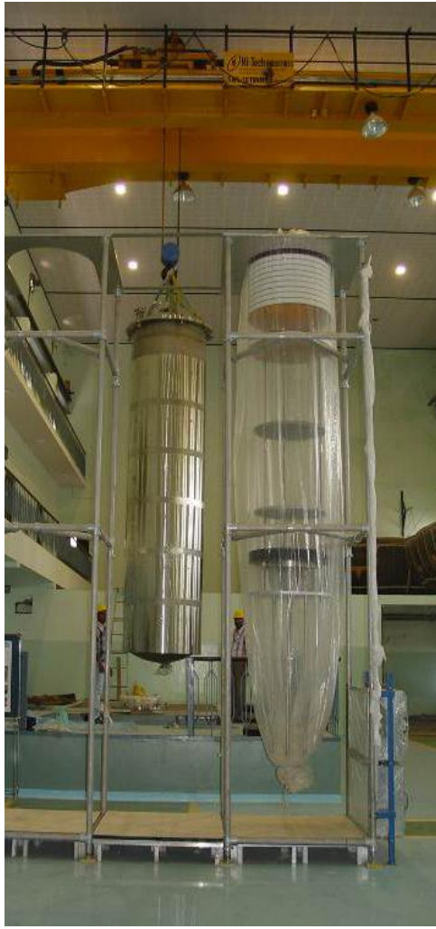
Cryostat & Cavity Insert Assembly
