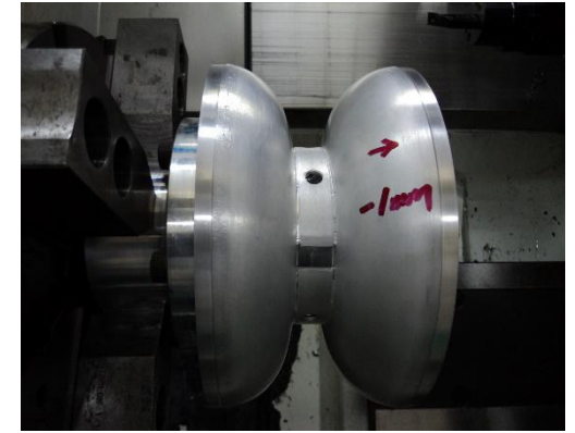
Machining of dumbbells on precision lathe
