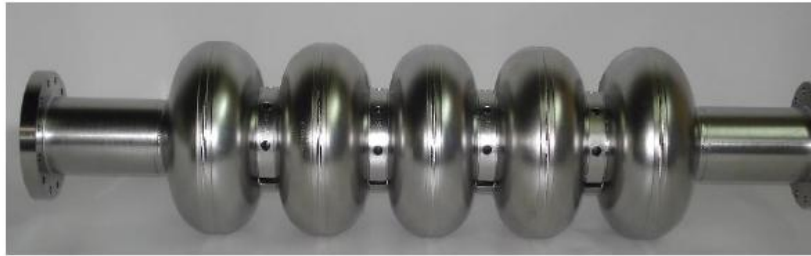
First multi-cell niobium cavity built in India
