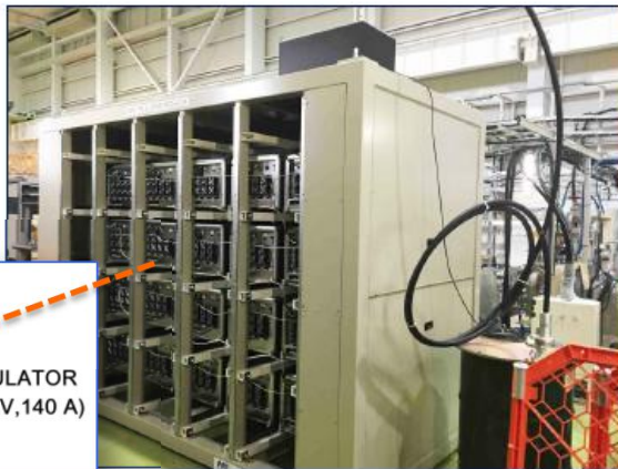
MARX modulator (20 Marx modules are used.)
