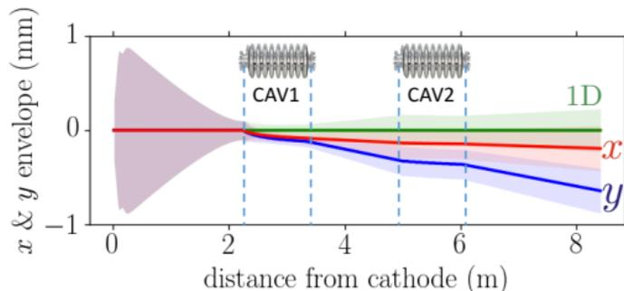
**Beam steering by the cavities has been experimentally observed**
