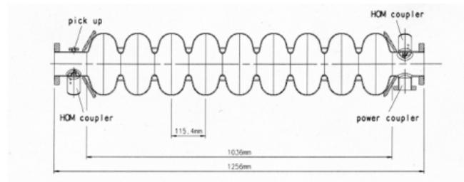
The transverse-focusing properties of such a cavity and non-ideal transverse-map effects introduced by field asymmetries in the vicinity of the input and high-order-mode radiofrequency (RF) couplers play a crucial role in transverse beam dynamics
