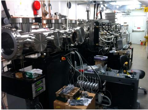
Figure 1: The APS Modular Deposition System incorporates in-situ metrology and an ion-beam figuring system for figure correction of mirrors up to 1.4 m long
