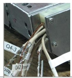
9 Beginning with any lead, cut the Expandable Sleeving (FC0053553) as needed to fully expose the Voltage Tap wire (F10050947). Using a soldering iron, heat the power lead so the solder melts and frees the Voltage Tap wire.
