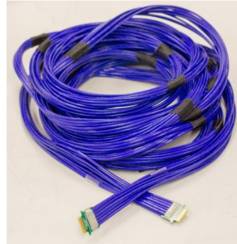
Cold data and LV cable: 7m long - one bundle of each per FEMB
