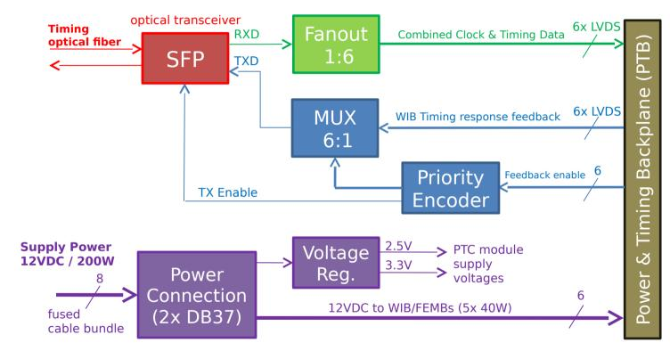
Note: 6 channels wired for SBND PTB backplane compatibility 5 channels used for ProtoDUNE
