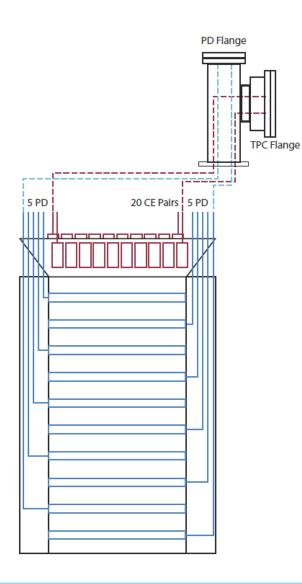
The PD cables for each APA are routed to a dedicated Feedthrough flange.
