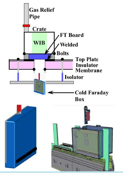
The signal ground of the FE ASIC is connected to the Detector Ground via the power returns in the warm electronics crate mounted on the top of the detector.
