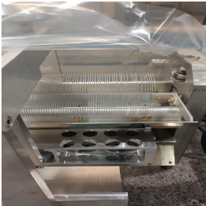
Replacing Broken Wires
