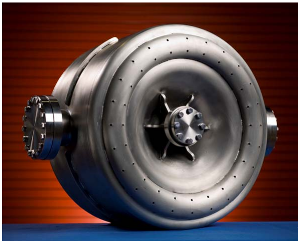
Figure 3.15: Photographs of the bare and dressed prototype SSR1 cavity
