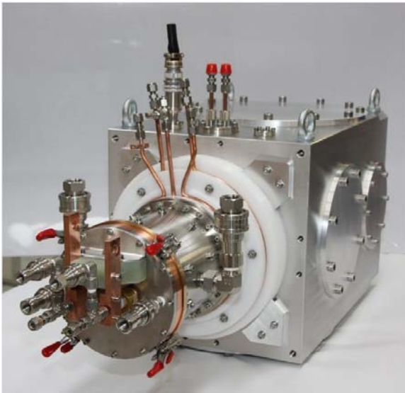
Figure 3.1: Photograph of the D-Pace ion source (foreground) with a vacuum chamber.
