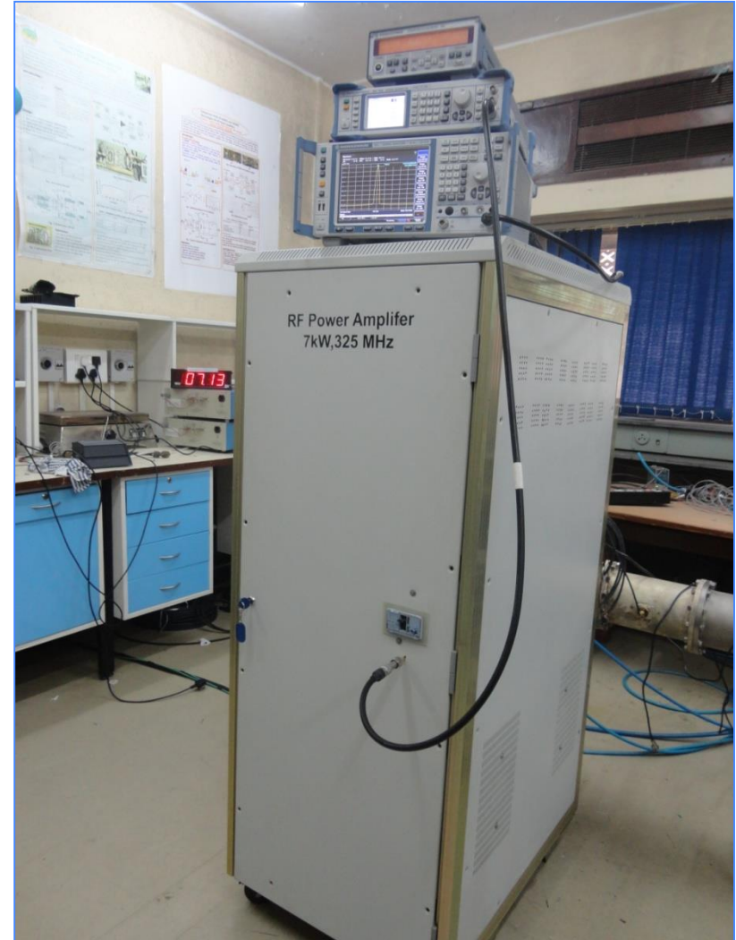
325 MHz, 7 kW Solid State Amplifier at BARC
