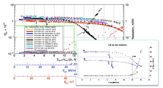
[1] Cold Tests of SSR1 Resonators Manufactured by IUAC for the Fermilab PIP-II Project, L. Ristori et. al, SRF15 Conference
