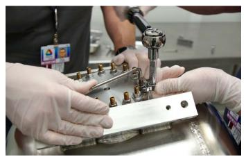
• The customized particle free procedure for SSR1 flanged connections ensures high reliability and avoids catastrophic damaging of cavity flange threaded holes (ED0004744)
