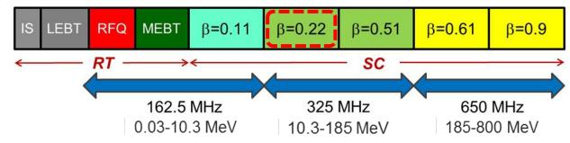
16 SSR1 cavities and 8 focusing lenses compose the two SSR1 cryomodules for PIP-II
