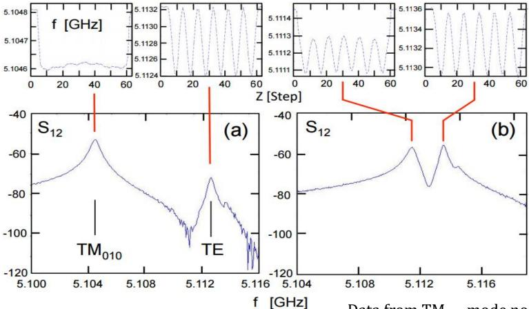
Data from  $TM_{010}$  mode no longer useful when mode is within  $\sim 3$  MHz of TE mode
