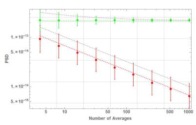
•Factor of 2 reduction in background spread, same improvement as doubling signal power by combining two cavities
