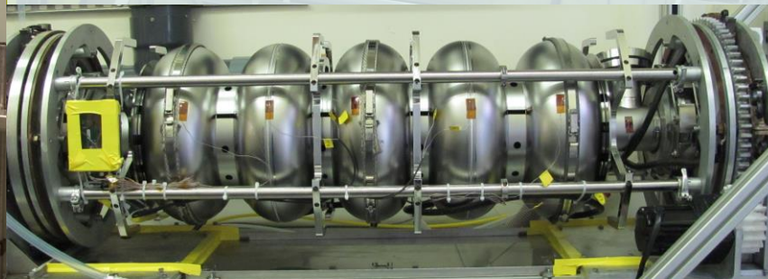
650 MHz Cavity Electropolishing
