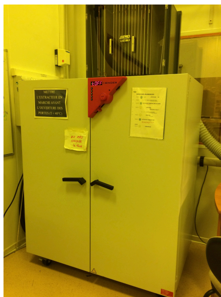
Heating chamber BINDER FED720
