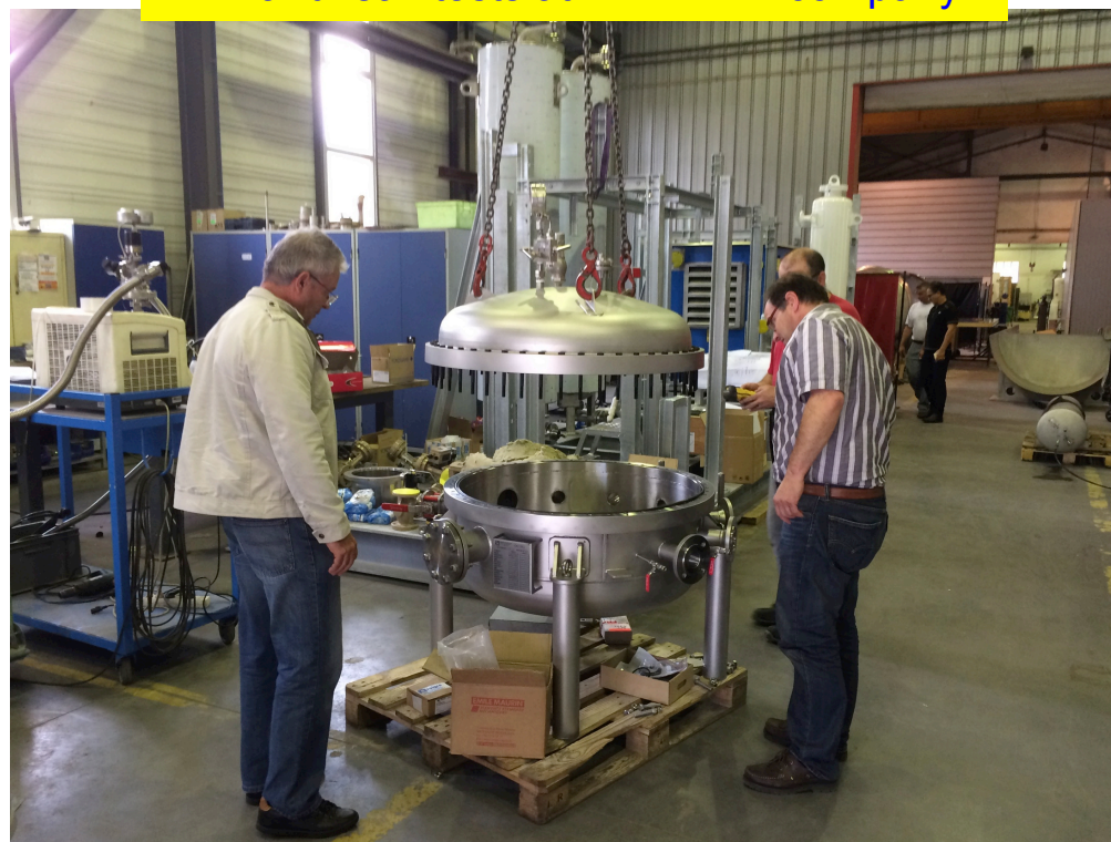
HP and leak tests at RAVANAT company
