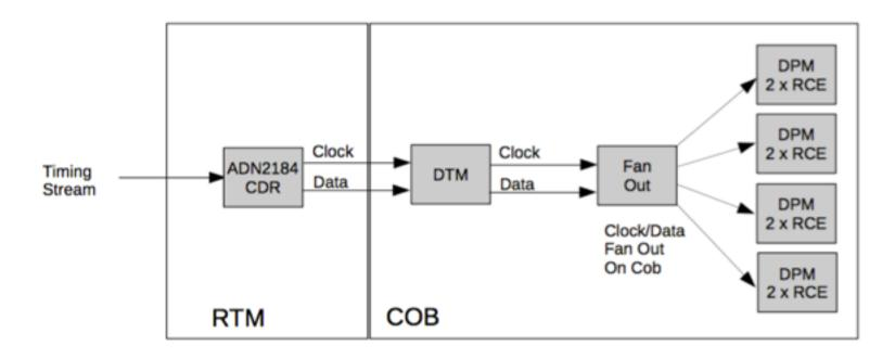
Clock and trigger/timestamp data separated on the RTM and sent to DTM which fans them out to each RCE (...this is really what the DTM is there for...)
