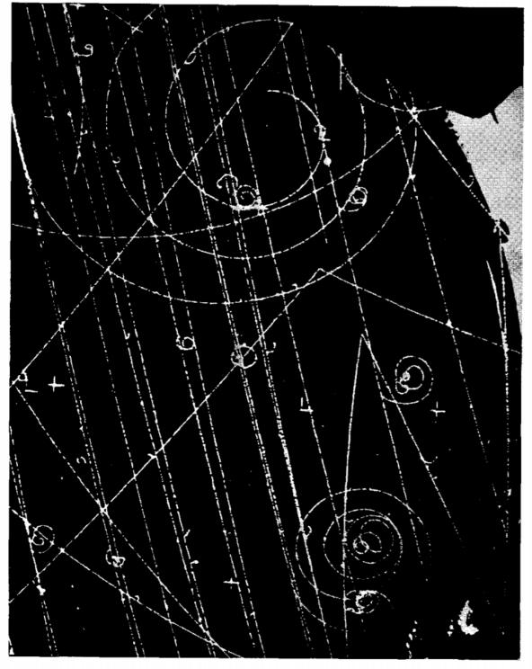
Fig. 1a A typical hydrogen bubble chamber photograph (Berkeley) with 1.1 BeV/c negative pions incident, showing an associated production.
