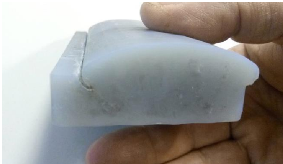
Clip mold 3D printed at CERN
