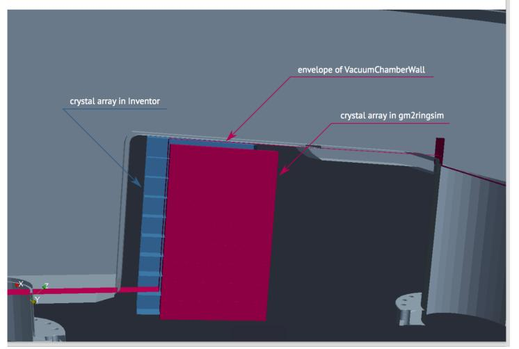
The Geant4 geometry built the chamber too large, relatively pushing the calorimeter farther back from the actual location.
