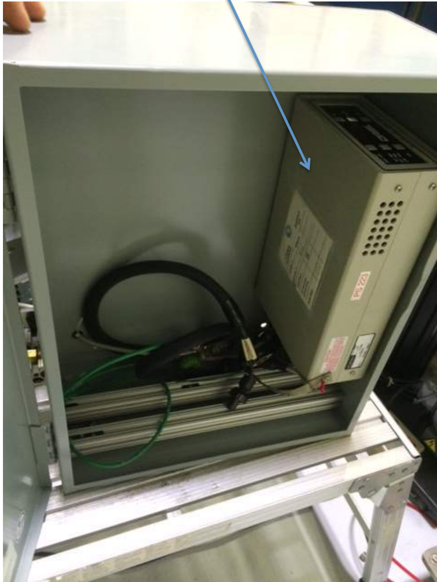
Light source power supply, shielded by an aluminum case, 24 V
