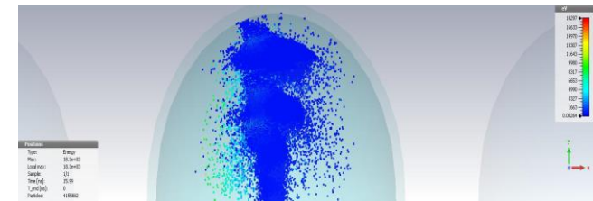
Particles after 16ns at Eacc=2.6MV/m (midcell)
