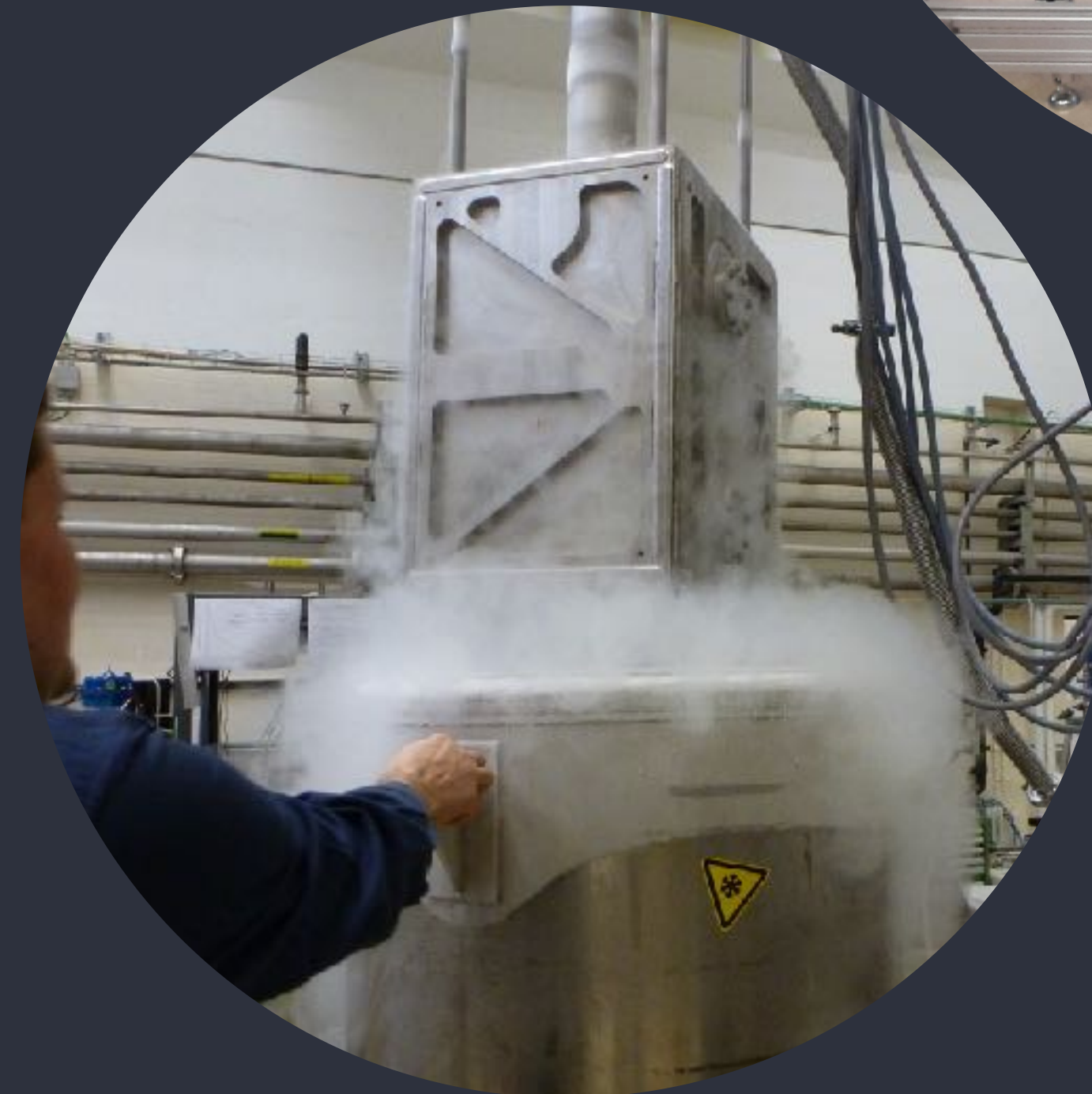
He-tank thermal shock test
