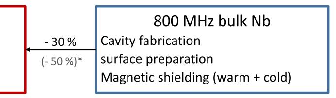
\* For seamless cavities and forming cost reduced by 50 %
