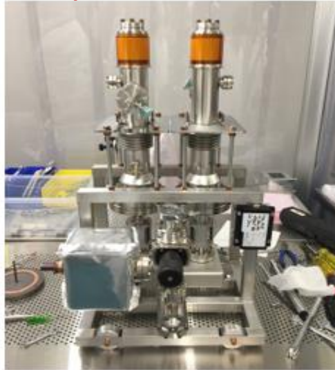
Assembling warm and cold pair for RF processing
