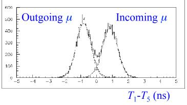
$\mu$  mass from TOF Fit to  $\beta$  vs  $p_{DC}$  gives  $m_{\mu} = 105 \text{ MeV}/c^2$
