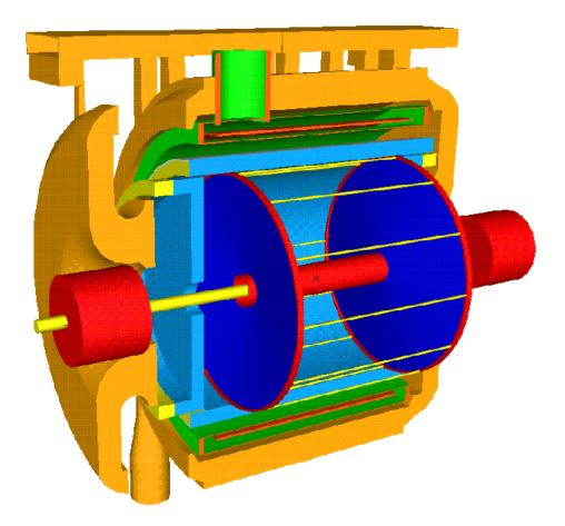
**Be beam pipe** (0.5 mm thick) **Instrumented permanent magnet quadrupoles** (32 PMT' s)
