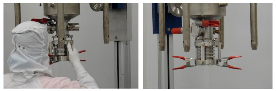
Extensive studies were done to choose the plate, gasket and spring clamp for the minimum particle generation
