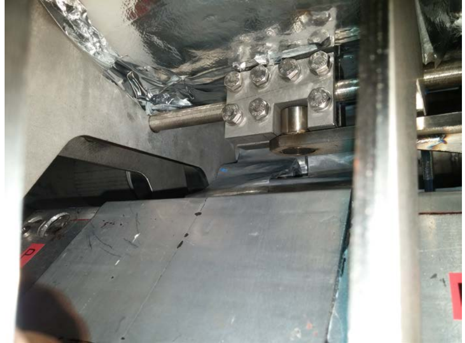
Reinforced clamp design for Cav#1 and Magnet for ProdCMs
