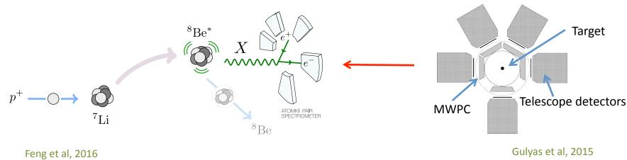
1.0  $\mu$ A proton beam from Van de Graaf generator impinge on LiF<sub>2</sub>, LiO<sub>2</sub> targets
