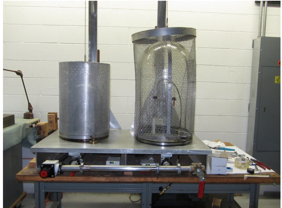
Setup for potting the resistors
