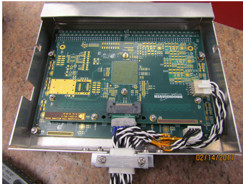
Box with cable clamp containing full FEMB assembly for cable routing and testing
