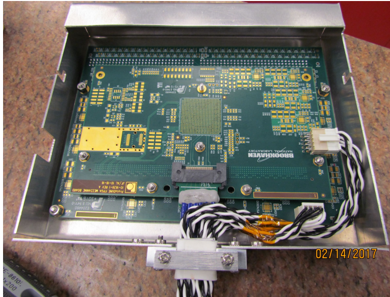
Figure 4: CE Box opened with an FEMB and expected cable routing inside the box.
