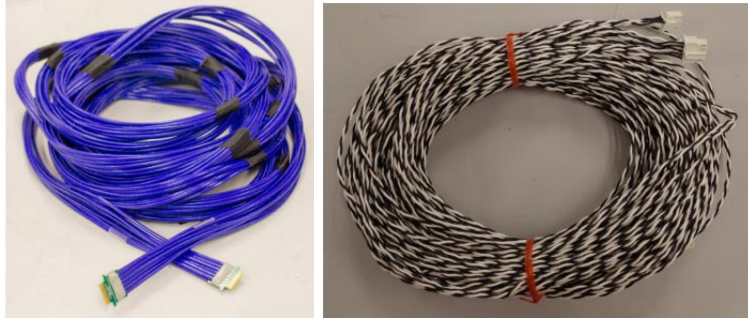
Figure 17: Prototype cold cable bundles; left: data; right: LV.
