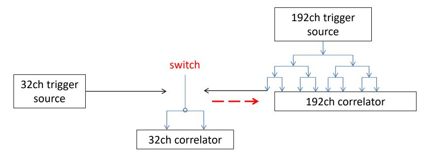
When powered on, the 32ch correlator initializes its ports – used to receive trigger signal – to high level. It behaves like a trigger signal and inversely triggered some of the chips on 192ch correlator unexpectedly.
