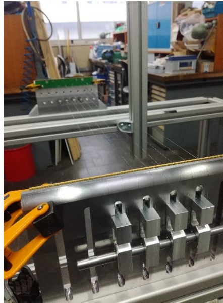
Pulleys and pulleys support for production tooling – Initial tension measurement
