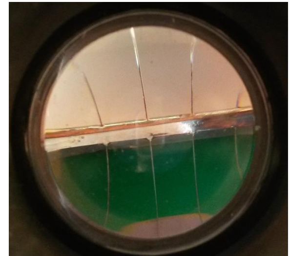
Test of grid brazing
