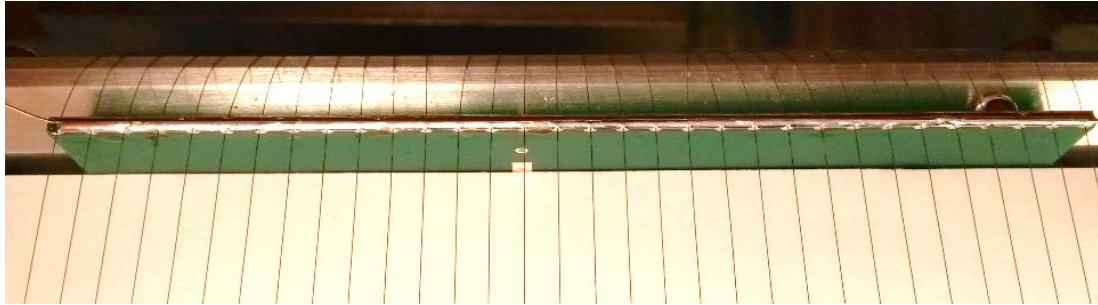
Test of grid brazing
